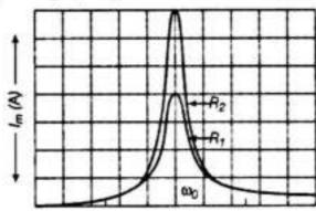
The condition for resonance in the L-C-R circuit is  $X_L = X_C$
