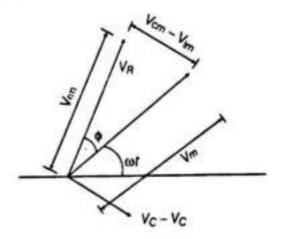
(iii) Impedance becomes minimum and equal to ohmic resistance
