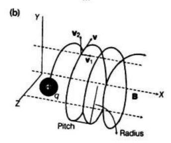
Component of velocity v parallel to magnetic field, will make the particle move along the field. Perpendicular component of velocity v, will cause the particle to move along a circular path in the plane perpendicular to the magnetic field. Hence, the particle will travel the helix path.
