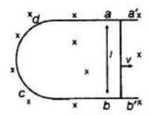
Let conductor shifts from ab to a'b' in time dt, then change in magnetic flux
