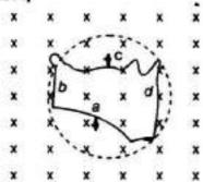
Ans. The wire is expanding to from a circle, which means that force is acting outwards on each part of the wire because of the magnetic field (acting in the downwards direction). The direction of the induced current should be such that it will produce magnetic field in upward direction (towards the reader). Hence, the force on the wire will be towards inward direction, i.e. induced current is flowing in anti-clockwise direction in the loop from chade.
